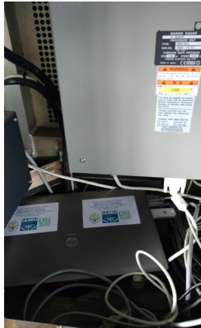
Fig. 5.3. a) The Furuno radar with ARPA on board the ship M/V Horyzont II b) the system for data registration
